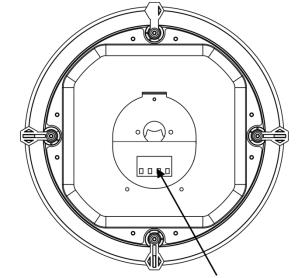
Connect the main feed cable (+) and the common cable (-)
