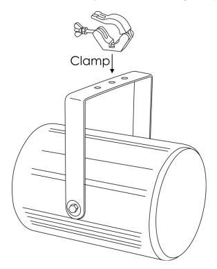
The PSU-620M can be mounted to any kind of truss with a clamp.
