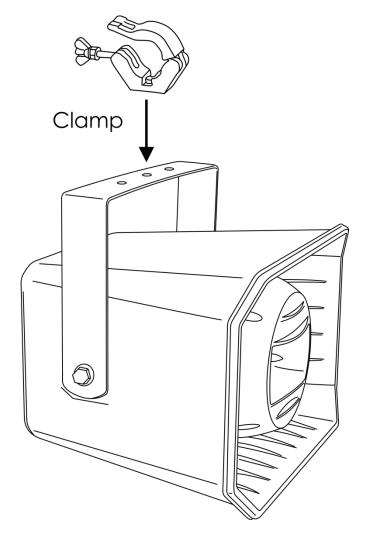
The MHS-50S can be mounted to any kind of truss with a clamp.
