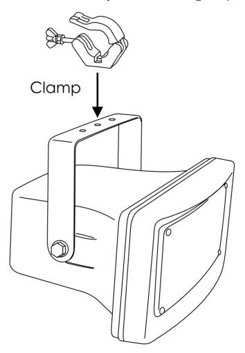
The MHS-30S can be mounted to any kind of truss with a clamp.
