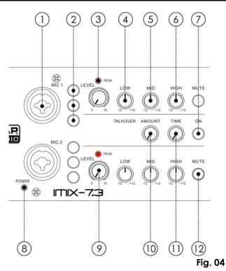
**01)** Mic balanced connector IN (mic 1/2) Electronically balanced combo-type input for connecting low impedance microphones. The input has extremely low noise and low hum. When connecting a microphone, make sure that the pin assignment is correct. Always make sure to read the manual of the microphone you want to connect. The XLR input is not suitable for connecting an additional mixing console, FX- unit, etc. You have to use the **line (54-58)** inputs, when connecting this kind of equipment.
