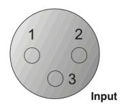
For unbalanced use PIN 1 and PIN 3 have to be bridged
