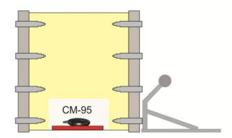
Make sure to place the CM-95 on a cushion, piece of isolation material or other soft material to avoid contact noise.
