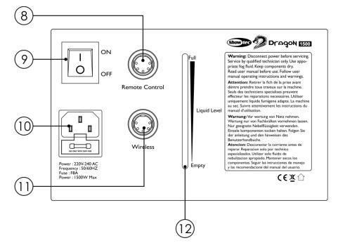
08) 5-pin DIN remote control connector IN
