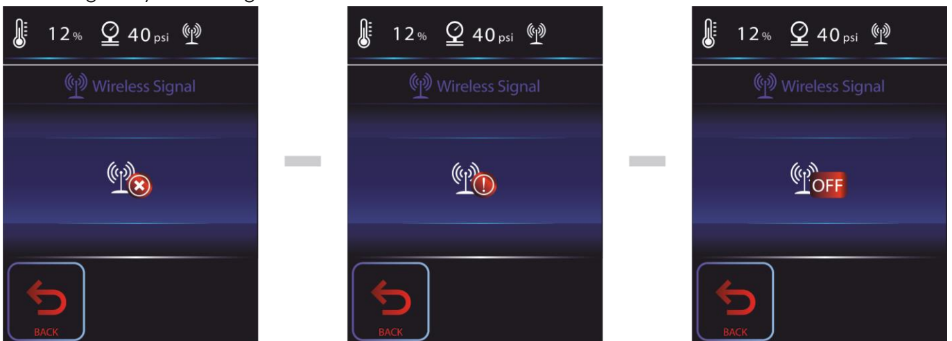
Problems wireless signal: W-DMX not assigned, No W-DMX signal or W-DMX Link lost (left to right)
