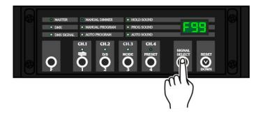
02) The adjustment range is between F00-F99, from 0 seconds to 10 seconds.
