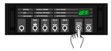
02) The adjustment range is between d00-dFF, from 0% intensity to 100% intensity.
