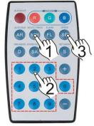
SP button (8): Press the speed button to activate the Running Speed function. This function is only available in color jump or color dream Mode. Use the + (13) and - (14) buttons to change the running speed. + = faster, - = slower
