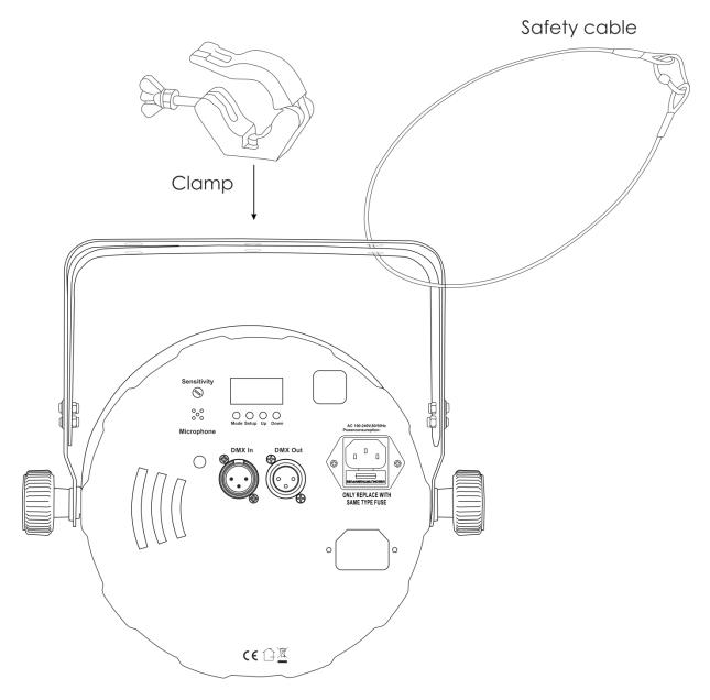
The Club Par 12-4 RGBW can be placed on a flat stage floor or mounted to any kind of truss with a clamp.
