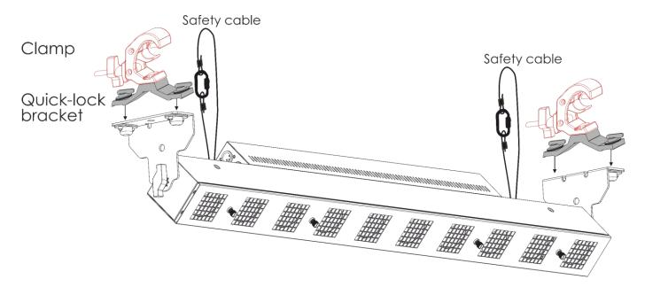
The Sunstrip LED can be placed on a flat stage floor or mounted to any kind of truss with clamps.
