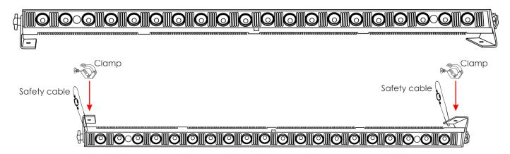
The Sunstrip II Stageblinder can be placed on a flat stage floor or mounted to any kind of truss with a clamp.
