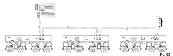
Note: Link all cables before connecting electric power!
