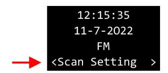
The settings menu is visible in the bottom line of the display.
