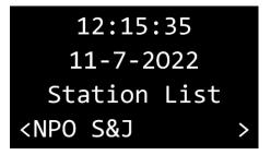
02) Press the PLAY/PAUSE button (D) to confirm. The device will activate the selected DAB+ radio station.
