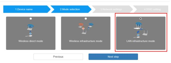
In this configuration the **built-in Wi-Fi** access point of the ALF-WirelessMedia **is disabled**:
