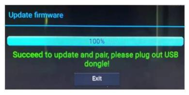
3. Plug out the dongle once the upgrading process is completed. Update all other dongles accordingly.
