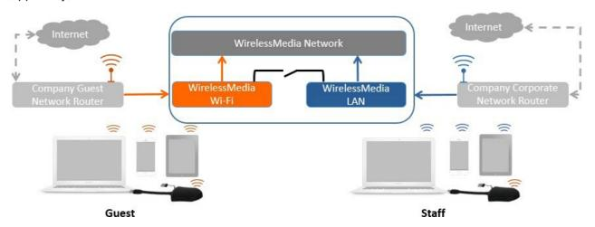
The dongle is connected to the Wi-Fi access Point of the Guest network, which in turn is connected to the internal Wi-Fi access Point of the ALF-WirelessMedia, the dongle can also be configured to connect to the enterprise's access point. Mobile users stay connected to their current network, have access to their normal corporate environment, as well as Internet access.
