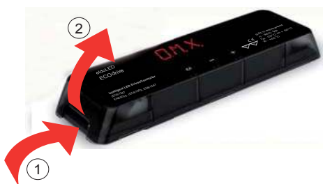
A Removing the cover
