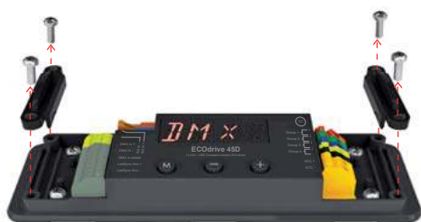
B Removing the strain reliefs
