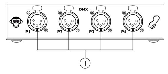
01) 4 x 5-pin DMX signal connector OUT
