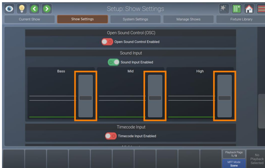
Fig. 61: Show Settings – Sound Input Signal Level
