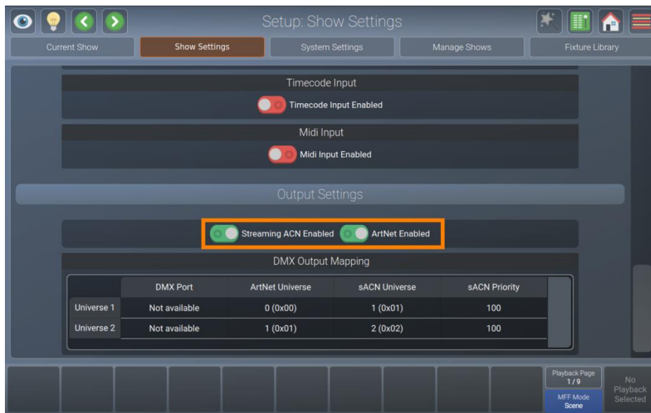
Fig. 64: Show Settings – DMX Output Configuration
