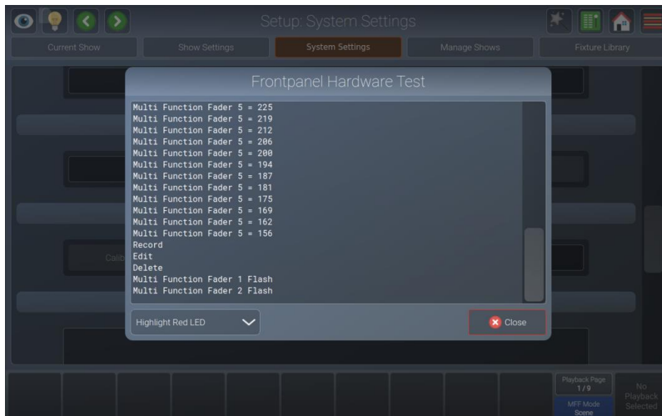
Fig. 74: System Settings – Front Panel Test dialog box
