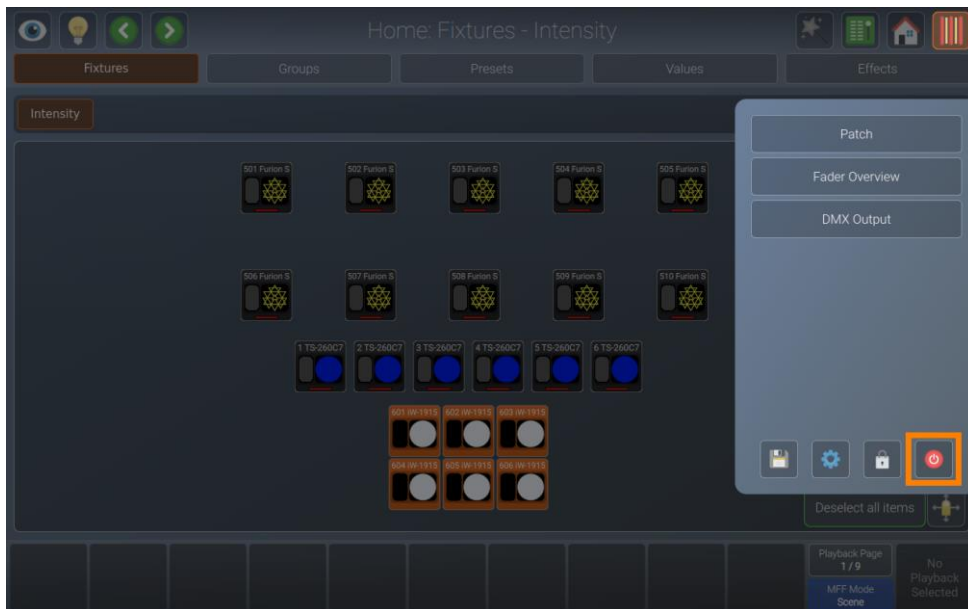
Fig. 185: Side Menu –Reboot / Shutdown Console
