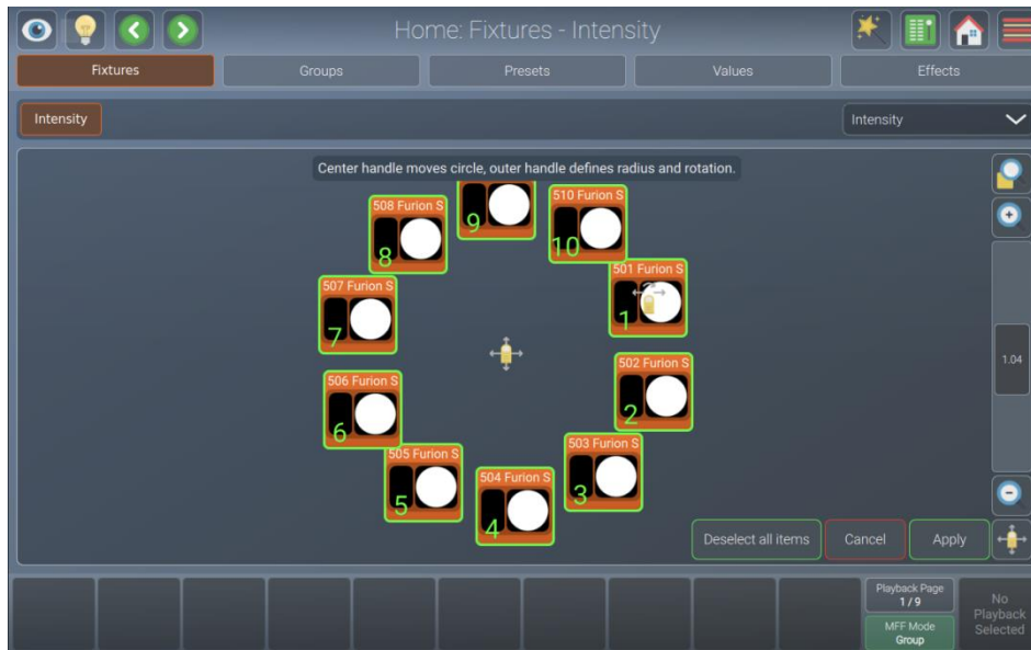
Fig. 97: Fixture View – Arrange Circular
